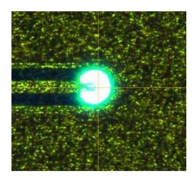
Kubos 25µm (radius) cubic GaN LED, with a quantum well peak in the 'green gap'
